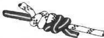
Figure 11 Double Fisherman's Knot
